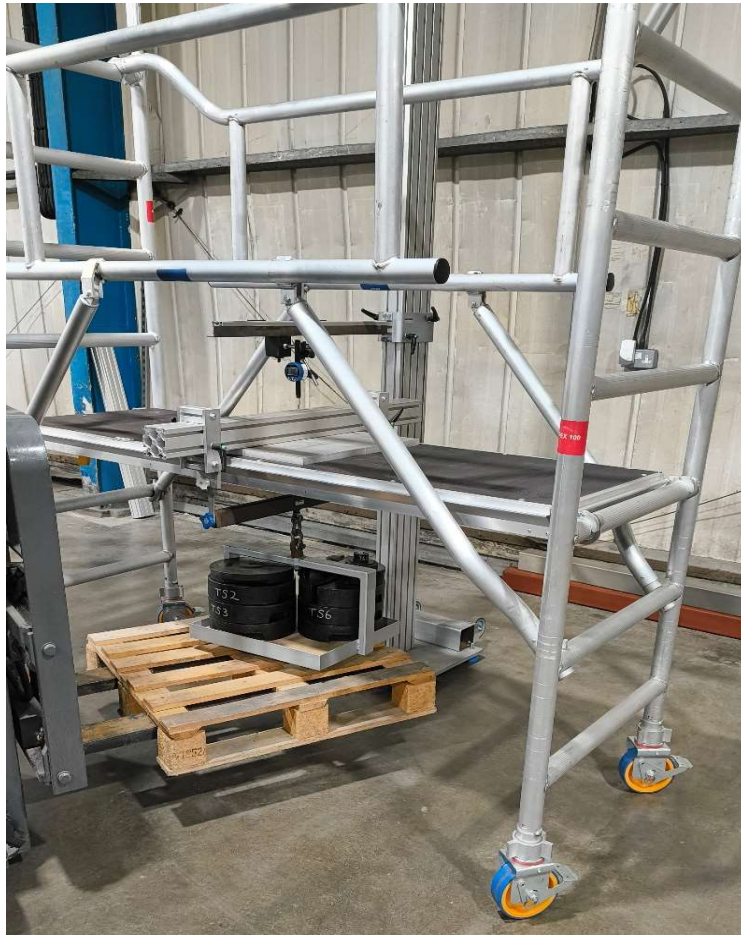
EN 1004-1 - 8.4.1. Elastic deflection of platform components
