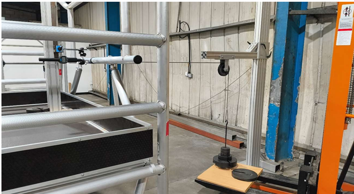
EN 1004-1 - 8.4.2. Elastic deflection of side protection
