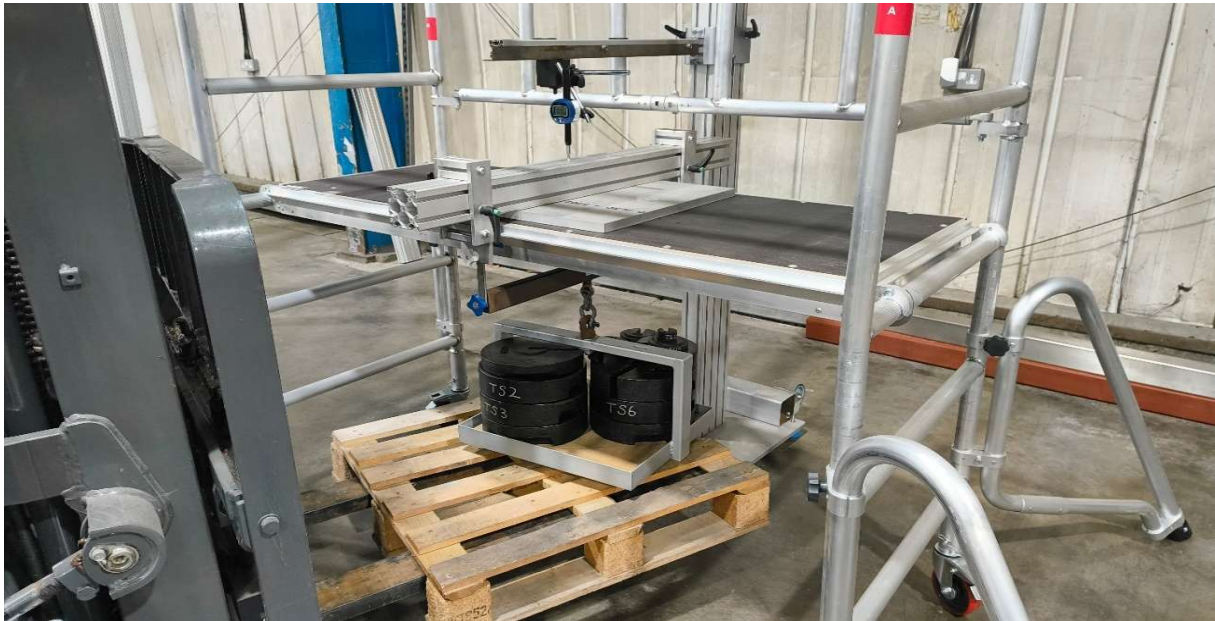
EN 1004-1 - 8.4.1. Elastic deflection of platform components
