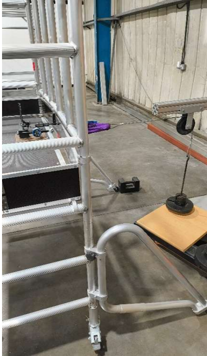
EN 1004-1 - 8.4.2. Elastic deflection of side protection (toeboard)
